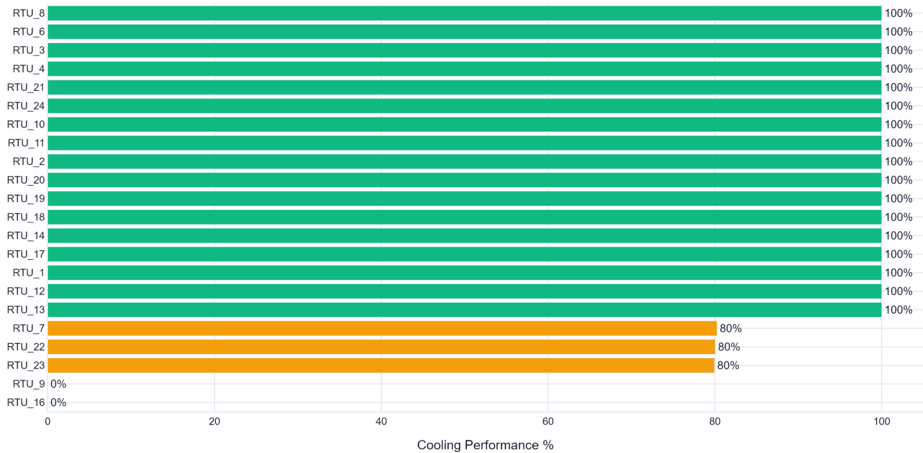
SAT Cooling Compliance - All RTUs
